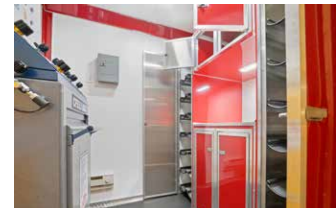
› The SCBA rack has spaces for 14 spare bottles. Cabinets can hold SCBA masks & parts, emergency provisions, first aid, Haz Mat, communication equipment, ropes and lines, and more. Recharge lights or phones, plug in the computer, do quick repairs.
